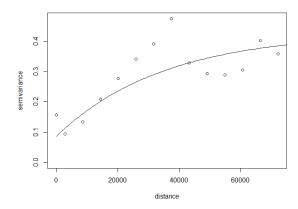
Figure 3: Empirical semivariogram plot based on all data available. The sill  $(\sigma^2)$ , range  $(\phi)$  and nugget  $(\tau^2)$  parameters can be estimated approximately from this plot around 0.37, 38000 and 0.08 respectively.
