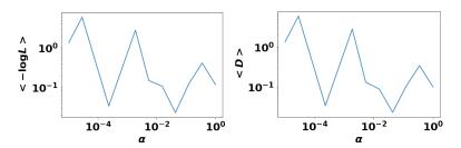
Figure 2: A parameter sweep over  $\alpha$  for the objective functions (6) and (7) to estimate the best hyper-parameter  $\alpha$ . The values plotted are the mean values over the validation set. The optimal value is  $\alpha \approx 4.3 \times 10^{-2}$ °.
